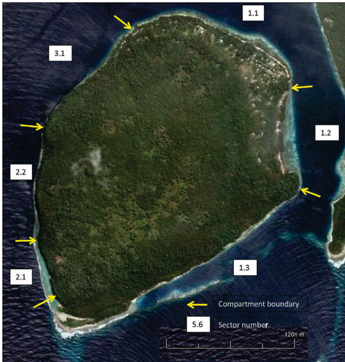
Figure 4.1 Example of coastal sectors recognised around a volcanic island: Luon, Solomon Islands.
