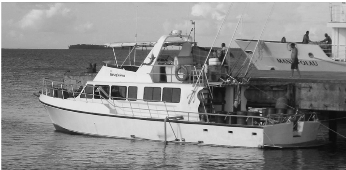
Figure 20. Photo showing the survey vessel Turagalevu. The mounting pole for the 8160 Multibeam echosounder transducer can be seen over the port side.
