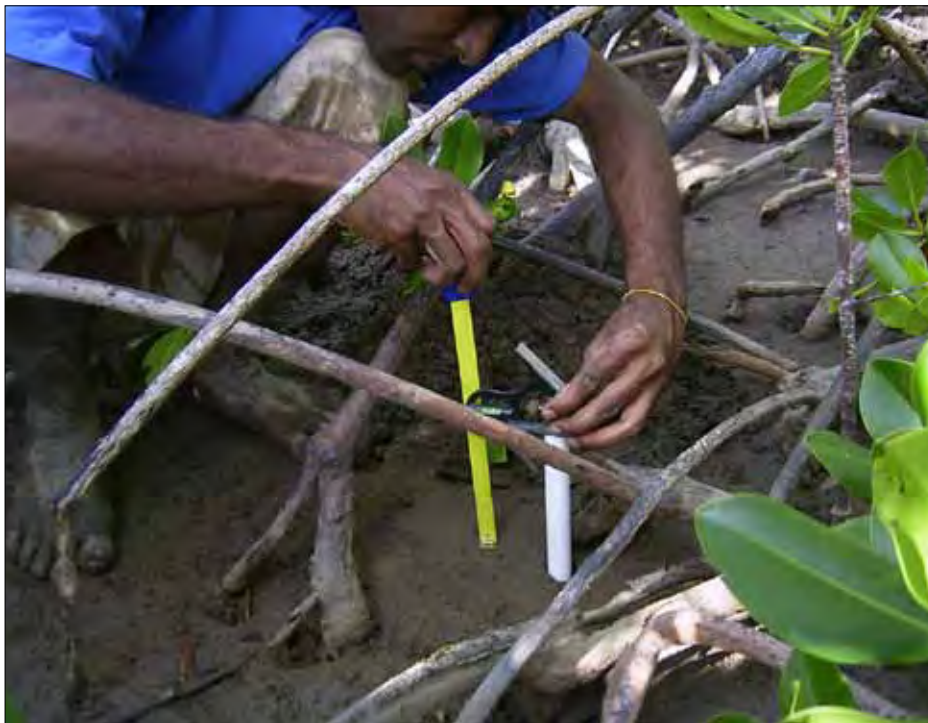
Figure 19. Sedimentation stake measurement at Tikina I Wai, Fiji
