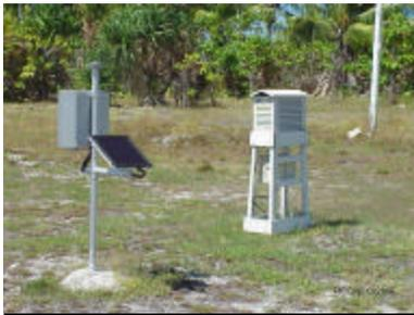
• Figure 19 A solar powered Automatic Weather Station
